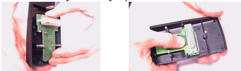
Figure 17: Adding the pwb into the MFJ-1
